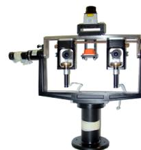
Figure 10. Stereo vision consistent of two Guppy monocular cameras mounted in a robotic head .
