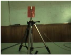
Figure 11. Right image acquired from stereo camera. The tracker sensor (with a white tape on it) is attached on a tripod for 3D point acquisition for calibration.
