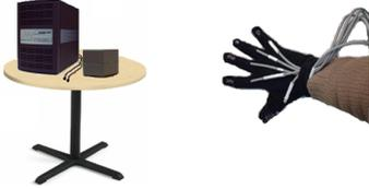
Figure 2. Polhemus Liberty tracker device and a glove with sensors attached on each fingertip.
