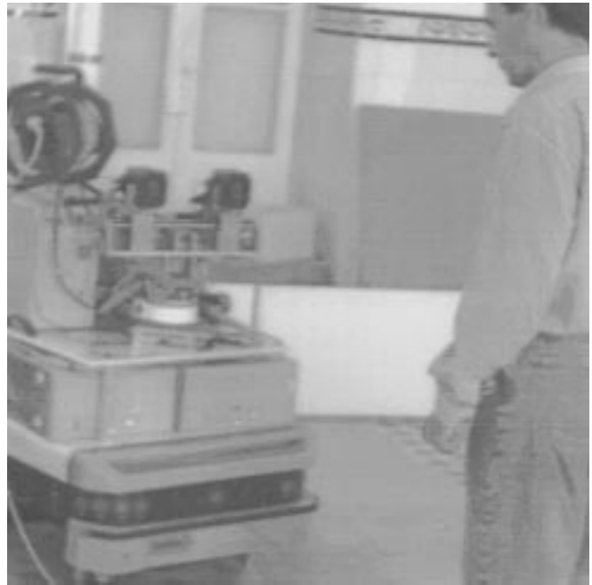
Fig. 1. The information provided by the active vision system is used to control the mobile robot to pursuit a person in real-time .
