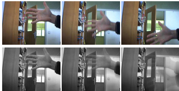
Figure 3: Example of background estimation. Top: input video sequence; bottom: resulting background image update
