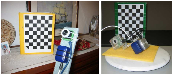
Fig. 8. Required setup for rotation calibration, and turntable used for translation calibration
