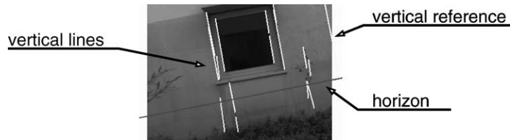
Fig. 2. Vertical line detection.
