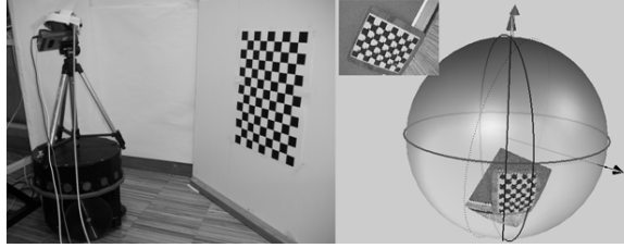
Fig. 6. Results of the calibration process: a) Calibration Set-up, b) Calibration Result (Unit Sphere projection)
