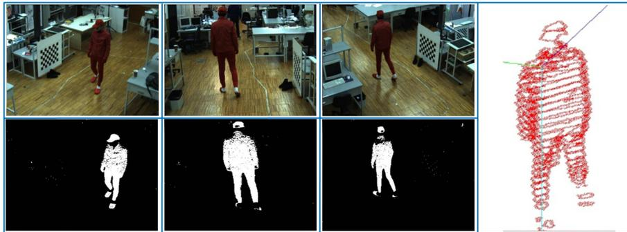
**Fig. 13.** Results of the 3D volumetric reconstruction of the person in the scene. The space is observed by a IS-camera network. Left pictures show the images of the person before and after background subtraction. The right image depicts the results of reconstruction. 35 inertial-based virtual planes, with an interval distance of 50 mm, are used for purpose of reconstruction.
