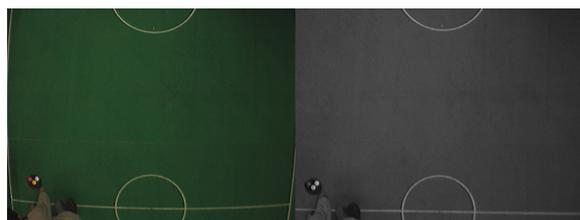
Fig. 10. Compound of two images: on the left, the original image having significant radial distortion; on the right, the radial distortion is corrected.
