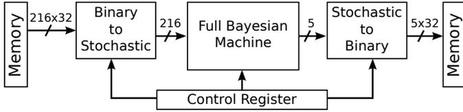
Fig. 2. Block diagram of the BM implementation.
