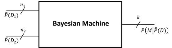
Fig. 1. Simple Bayesian Machine with two inputs and one output, and no free variables. The compilation toolchain takes a Bayesian program specification and uses ProBT to have a symbolic description of the computation used to synthesise the machine.
