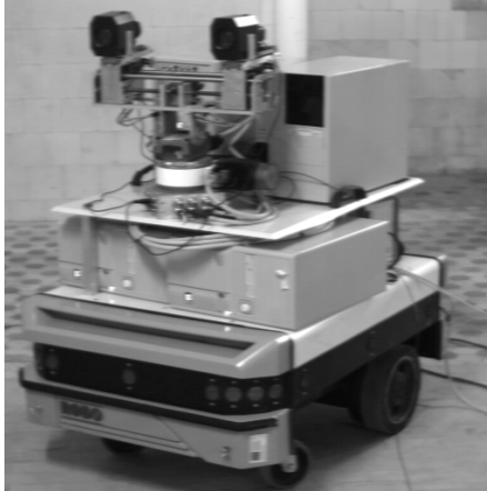
Fig. 6. The active vision system and the mobile robot.
