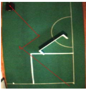
Figure 5: Overview of the reactive obstacle avoidance test. The red line denotes the robot trajectory in the experiment.
