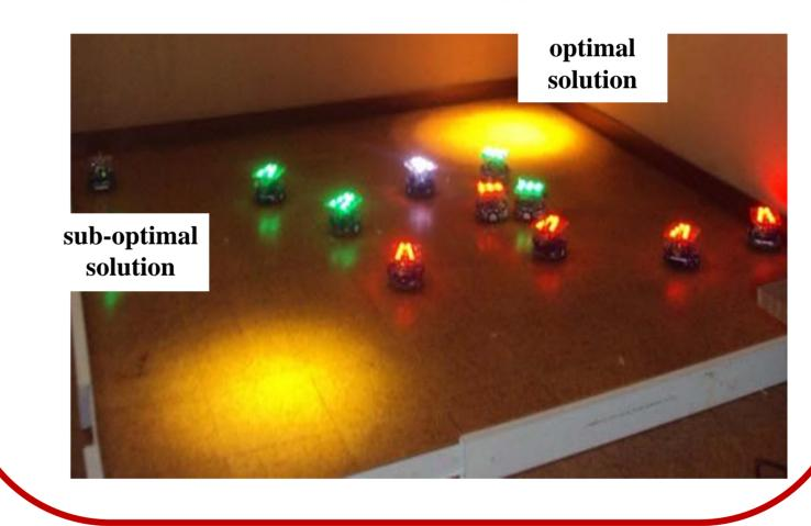
Preliminary results show that, with both simulated and physical robots, the global optimum is achieved in approximately 90% of the experiments
