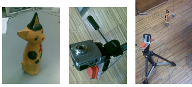
Figure 6. Left: Cat statue, Middle: Couple of camera-IMU sensor, Right: A snapshot of the scene.
