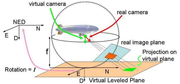
Figure 3. The virtual leveled plane concept.
