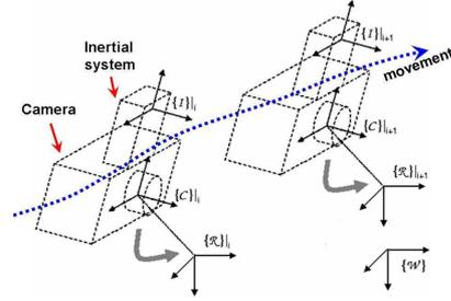
Figure 2. Definition of frames of reference.
