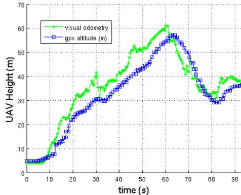
Figure 10. Visual odometry based on homology compared with GPS altitude measurements.
