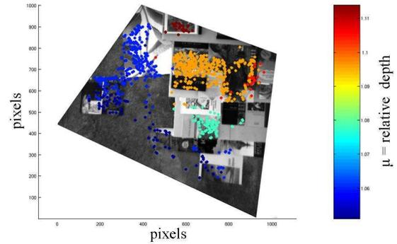
Figure 9. The relative depths from two views used to order planes by their height.
