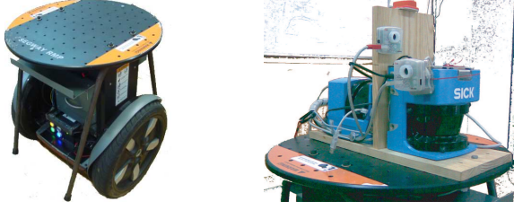
Fig. 7: The sensor platform comprising of two laser range finders and two cameras is mounted on the Segway RMP 200.
