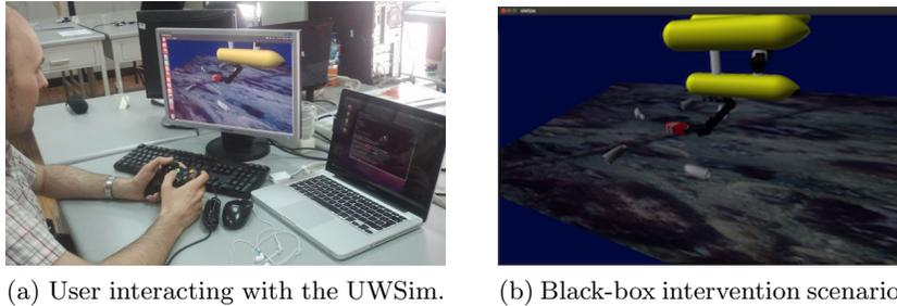
Fig. 7: User interaction with the UWSim simulator using a gamepad controller to train the system. The user gets complete 3D visual information and contact feedback from the observed scene.
