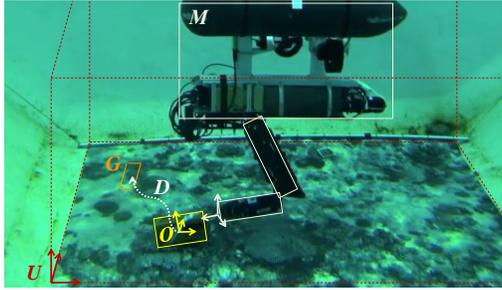
Fig. 3: Underwater intervention scenario. A manipulator  $M$  detects and object  $O$  in a workspace  $U$ . Upon a user specified goal  $G$  (or task), it should be capable of, autonomously, estimate a solution  $D$  for successfully accomplish its mission.
