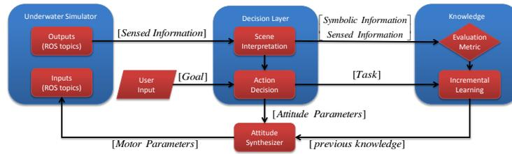
Fig. 9: Execution and Incremental Learning Block Diagram.
