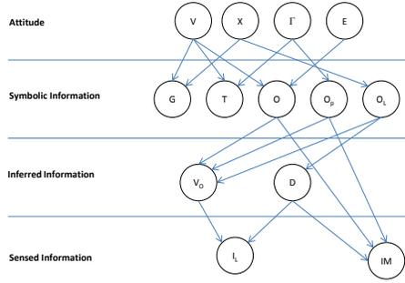
Fig. 5: Directed Acyclic Graph of the proposed Dynamic Bayesian Network. Nodes represent variables and directed arcs represent variable dependencies.
