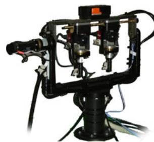
**Fig. 7** View of the current version of the Integrated Multimodal Perception Experimental Platform (IMPEP). The active perception head mounting hardware and motors were designed by the perception on purpose (POP—EC project number FP6-IST-2004-027268) team of the ISR/FCT-UC, and the sensor systems mounted at the Mobile Robotics Laboratory of the same institute, within the scope of the Bayesian approach to cognitive systems project (BACS—EC project number FP6-IST-027140)
