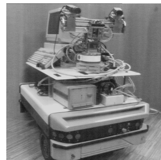
Figure 1: The mobile system with the active vision system.
