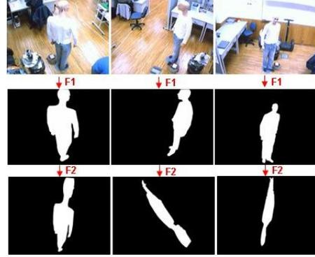
Figure 6: From real image planes to virtual image planes: F1: Background subtraction process. F2: Image plane of virtual camera.
