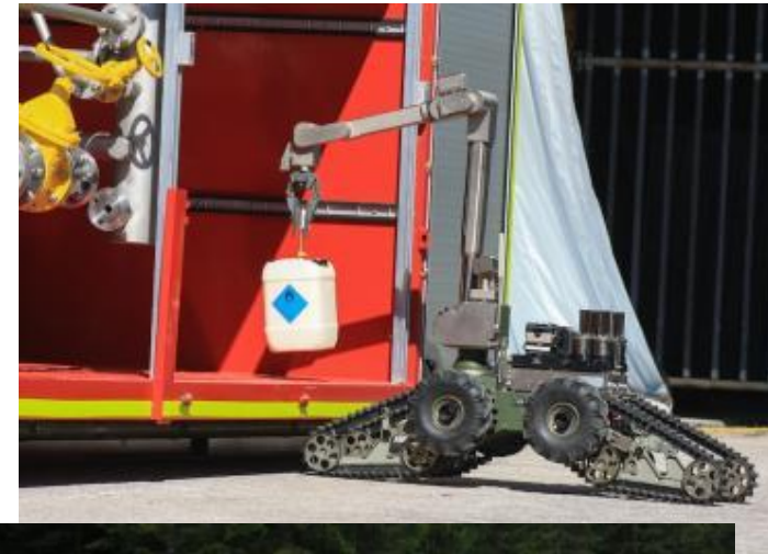
Manipulation of hazardous materials
