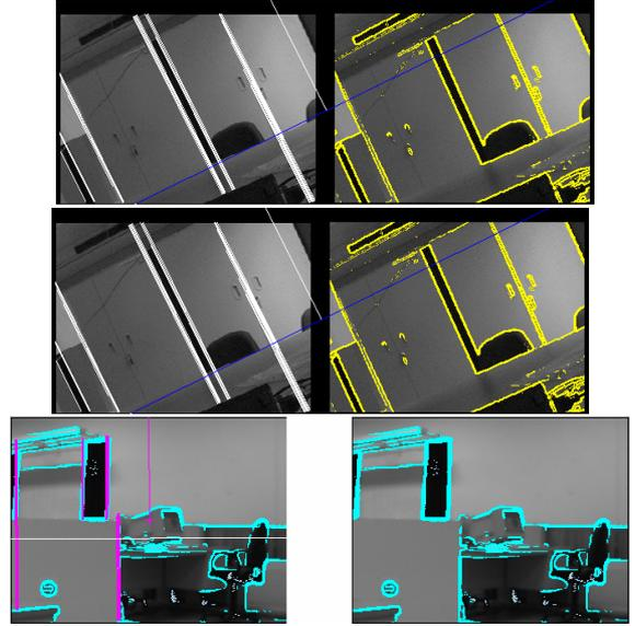
Figure 8: Detected vertical lines.
