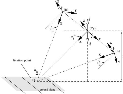
Figure 10: Ground plane point fixated. The point  $\vec{P}_f$  in the ground plane is visualised by the active vision system. The geometry of this visualisation corresponds to a state, named visual fixation.
