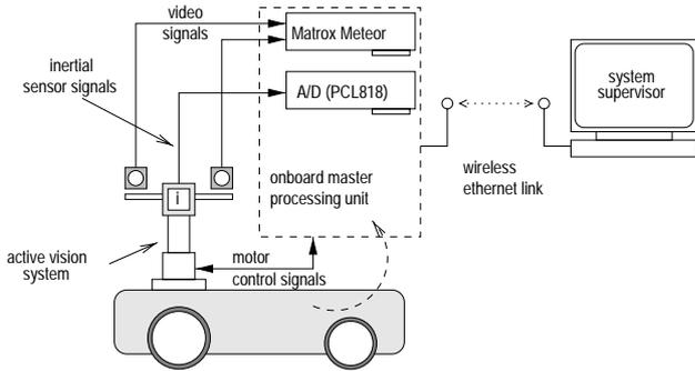
Figure 5: System Architecture. The inertial system processing board uses the Master processing unit as host computer.
