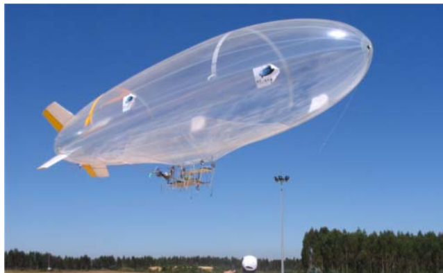
Fig. 2. The aerial vehicle instruments include a vision system and a low-cost inertial measurement unit.
