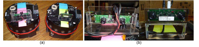
Fig. 3. Mobile robots used on the 3-D mapping experiments: (a) Scout mobile robots from Nomadic Technologies; (b) stereo-vision sensors from Videre Design mounted on the robots. Both robots have colored markers on the top, in order to compute their pose in a global reference frame \{W\} , through a RGB camera covering the robots’ workspace and color segmentation.
