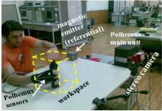
Fig.2. Experimental setup for single hand exploration.
