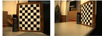
Fig. 3. Two examples of calibration images used to calibrate the camera-inertial system.
