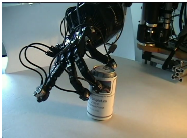
Each Finger is stopped independently when contact is detected
