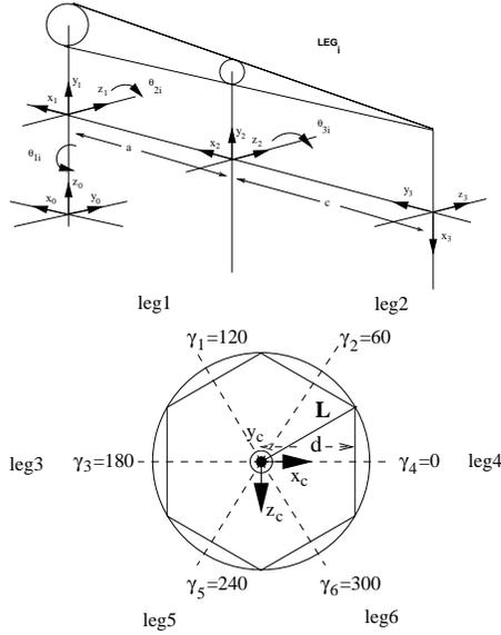
Figure 2: The coordinate systems defined for each leg. Legs' locations around the central body.
