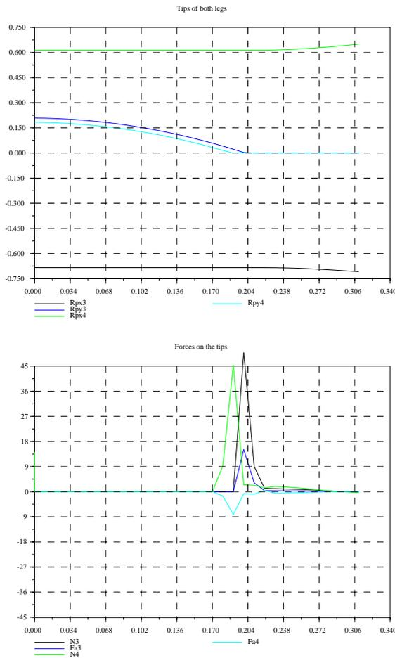
Figure 7: Graph1: Evolution of tips position of both legs in inertial frame (Position(m) versus Time(s)). Graph2: Applied forces on the tips of both legs (Force(N) versus Time(s)).
