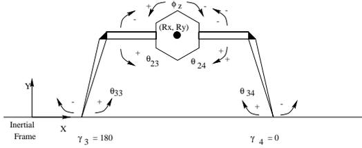
Figure 3: Independent variables of 2D kinematic model.
