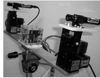
Fig. 7. Stereo camera rig with IMU based on low cost sensors.
