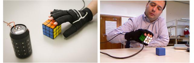
Fig. 4. Experimental setup used: a glove with distributed accelerometers (Acceleglove[5]), and instrumented objects, cube and soda can, with tactile and inertial sensors [3]; and example of performing a grasp.
