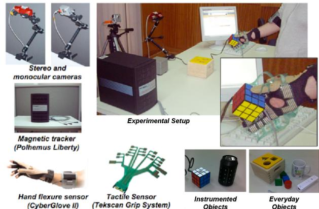
Fig. 1. Global overview of the HANDLE experimental area, data acquisition devices and objects available [3].
