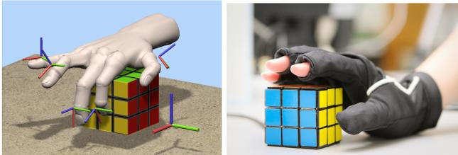
Fig. 2. Accelerometer sensor sensor axis distributed on the hand and object, and actual instrumented object and glove with the accelerometers.
