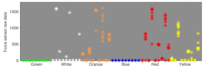
Fig. 5. Overlay of tactile force distribution on the instrumented cube during manipulation, 9 sensing cells per coloured face.
