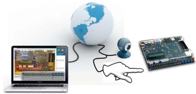
Figure 1. Basic concept of the reconfigurable logic remote lab: control the board switches and keys and look at the development board.
