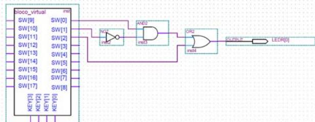
Figure 5. Simple combinational circuit using virtual block.
