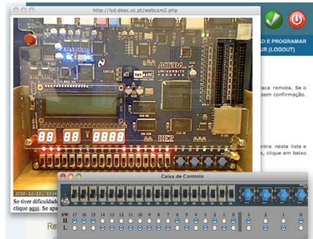
Figure 2. Screen shot of the remote laboratory interaction with the FPGA board.
