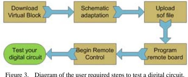
Figure 3. Diagram of the user required steps to test a digital circuit.
