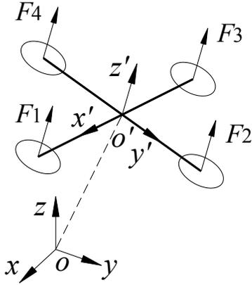
Figure 2. Quad-rotor UAV coordinate systems
