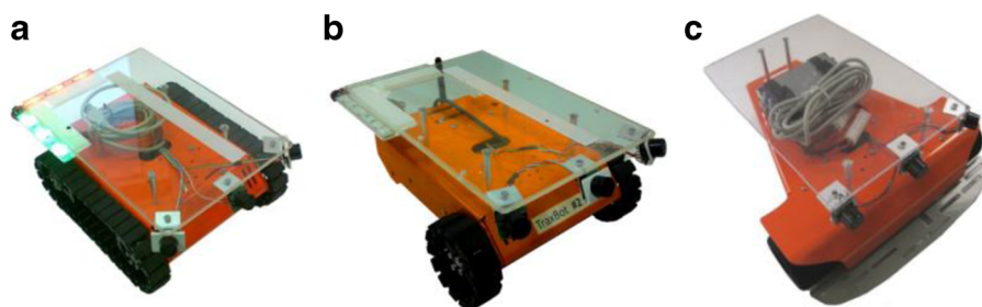
Fig. 3 Arduino-based robotic platforms, a TraxBot v1; b TraxBot v2; c StingBot
