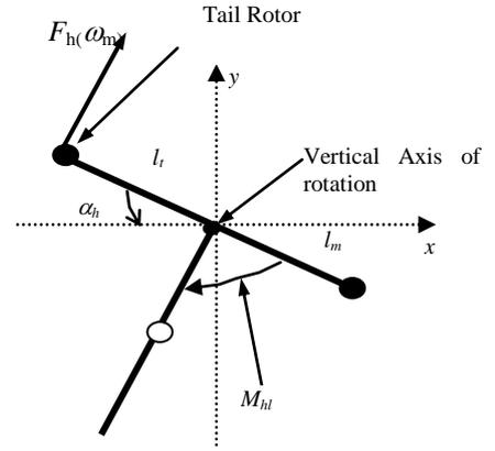
Fig. 5. Moments of forces in horizontal plane.
