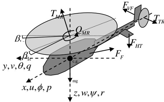
Fig. 10. Forces in the Real Helicopter.
