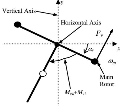
Fig. 4. Propulsive force moment and friction moment in the TRMS.
