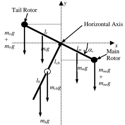
Fig. 3. Gravity forces in the TRMS, corresponding to the return torque, which determines the equilibrium position of the system.
