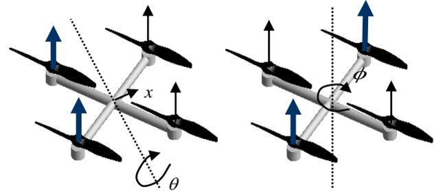
Fig. 7. Forces resulting from the movement in the  $x$ -axis around  $z$ -axis.
