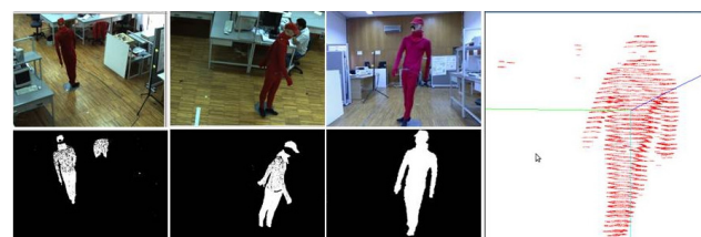
Fig. 19 Result of 3D reconstruction when a mobile sensor is augmented to the network (corresponding to Fig. 18); In order to have more details of the scene, a mobile sensor is navigated close to the manikin and its view is integrated as a new node in the network. The left two columns are the images corresponding to the two fixed cameras and the third column from left is the image corresponding to the mobile camera. The results of the 3D reconstruction by using two fixed IS-camera couples and a new augmented couple are demonstrated in the right column.
