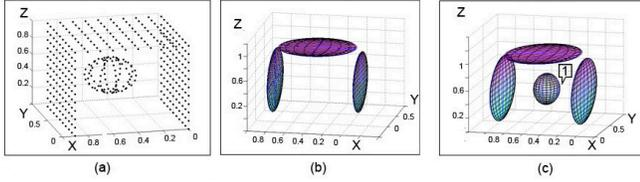
Fig. 3. Novelty detection algorithm: a) ideal 3D corridor where an object was placed inside; b) GMM associated to the corridor map; c) GMM associated to a). The novelty detected by the algorithm has been indicated by the label '1'.
