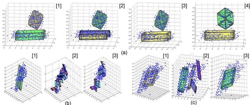
Fig. 6. Testing the 3D shape retrieval algorithms using superquadrics with simulated data (a) and real data (b-c).
