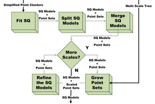
Fig. 4. Data flow of the 3-D shape retrieval using superquadrics. The black arrows represent the input (simplified point clusters and multi-scale tree) and the output (superquadric models).
