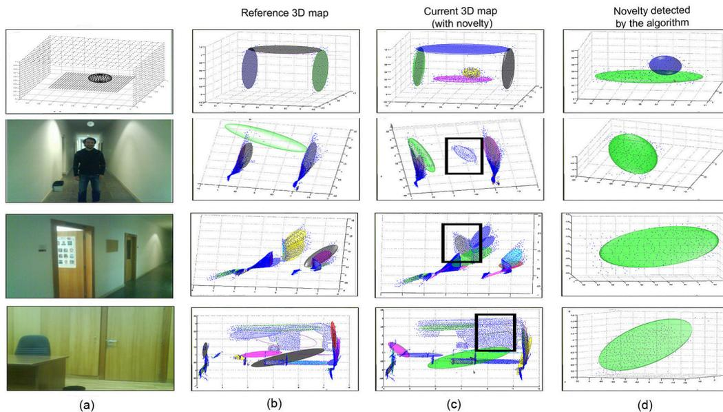
Fig. 5. Testing the change detection algorithms, where the first row represents simulated data, the others are real data. a) Photos of the testing sites with novelties; b) reference 3D map; c) the current 3D map including the novelty (black boxes); d) detected changes, with "zoom" in the novelty.
