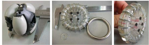
Fig. 11. Plastic omni wheel used in conveyor belts and omni wheel built from standard parts and machined acrylic.
