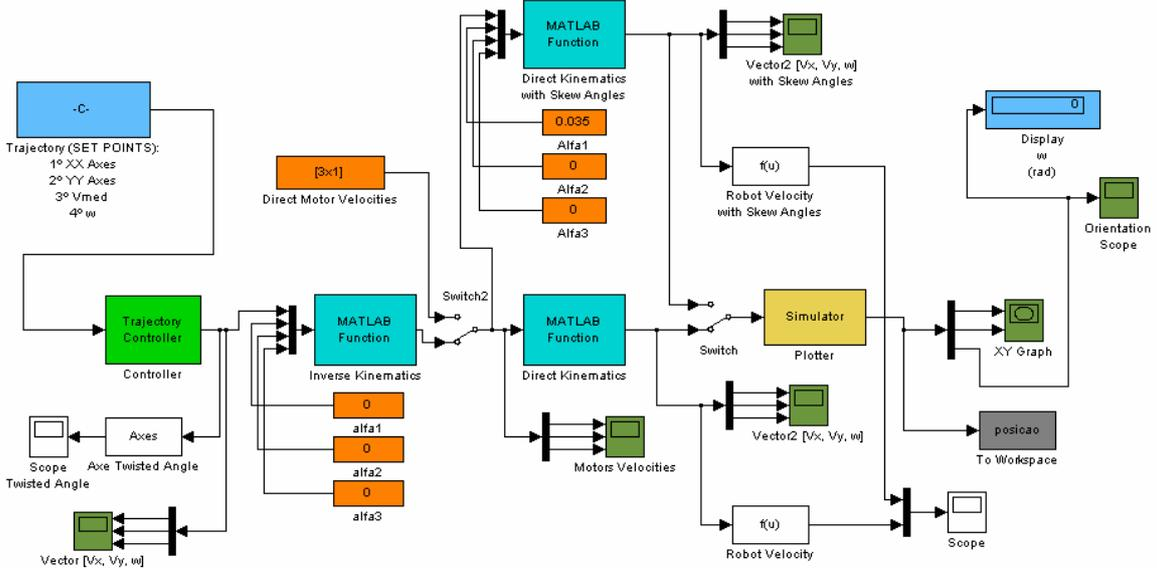
Fig. 5. Controller model and motion simulator.
