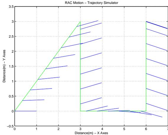
Fig. 6. Robot trajectory following set points  $(3, 3, 10, 05)$ ,  $(3, 0, 1, 0)$ ,  $(6, 0, 1, -0.15)$ ,  $(6, 3, 1, 0)$  considering ideal robot geometry.
