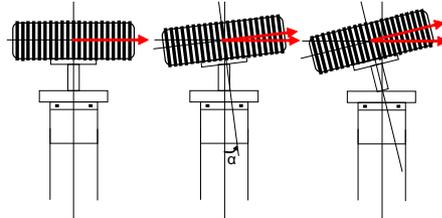
Fig. 8. Wheel skew angle.
