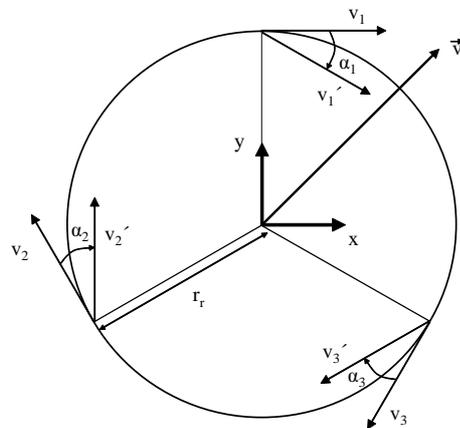
Fig. 4. Illustration of robot kinematics for tangential and twisted assembly of wheels.
