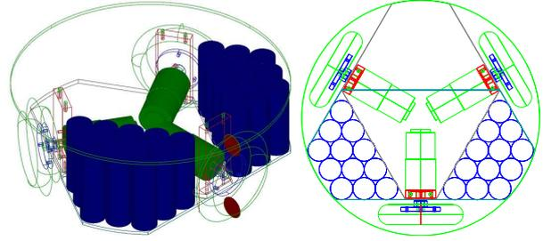
Fig. 10. *RacBot* chassis and motor drive layout.
