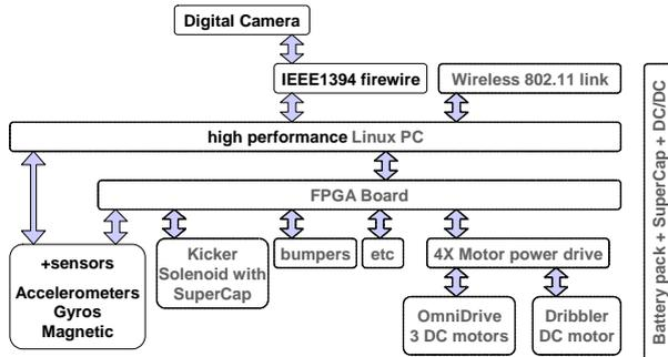
Fig. 3. *RacSmartBots* - enhanced robot implementation.
