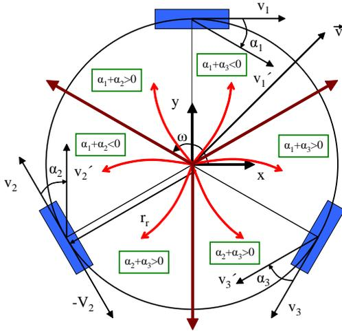
Fig. 9. Skew wheels angle relation to different trajectories.
