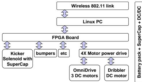
Fig. 2. *RacSlaveBots* - basic robot implementation.
