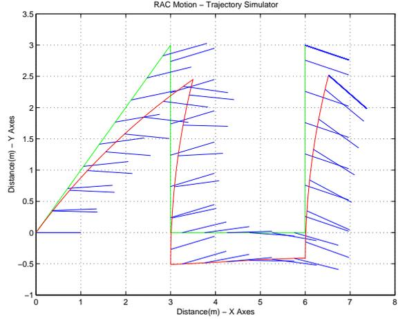
Fig. 7. Robot trajectory with unknown skew angles (red), and correct robot trajectory with calibrated skew angles (green).
