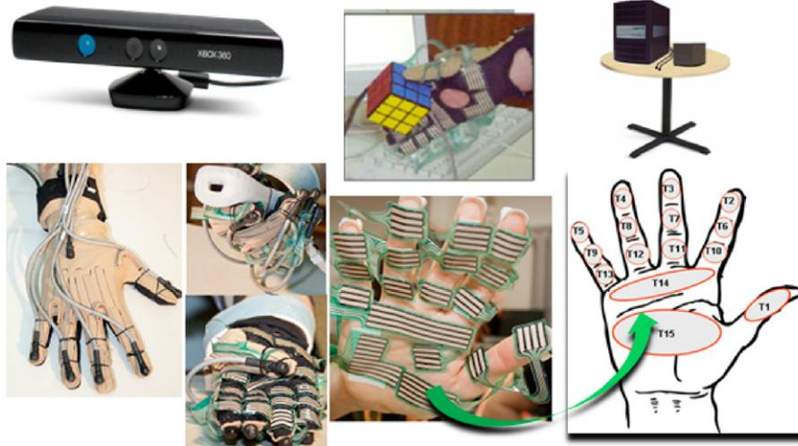
**Fig. 11.** Sensors used in our experimental setup: RGB-D camera (MS-Kinect), Polhemus Liberty Magnetic Tracking System, Cyber-Glove and Teksan Tactile sensors.
