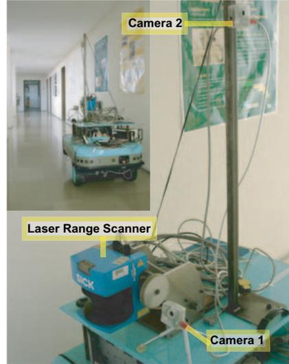
Fig. 3. The Robuter mobile robot platform with two cameras and a Laser Range Finder.
